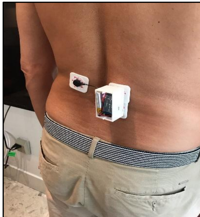
Figure 2b: sEMG sensors were placed at the lower erector spinae.
