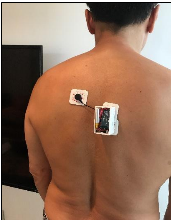
Figure 2a: sEMG sensors were placed at the middle trapezius.
